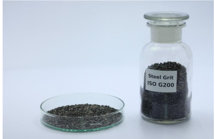
High Carbon Cast Steel Grit ISO G200 (SAE G12)
