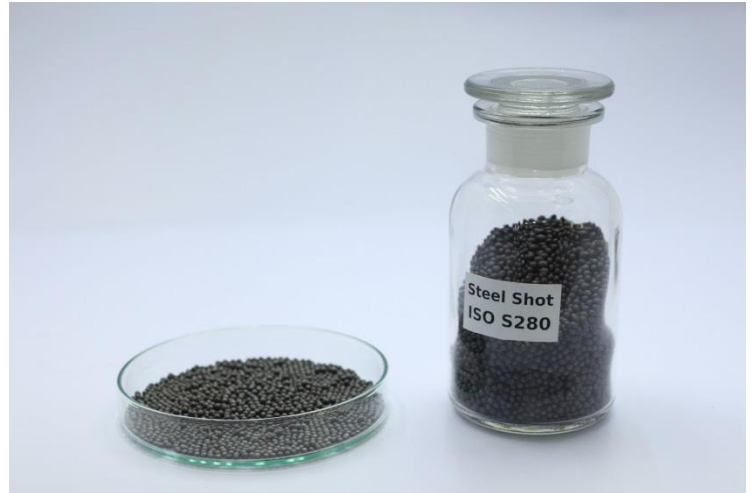
High Carbon Cast Steel Shot ISO S280 (SAE S930)
